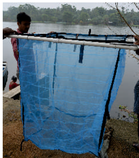
Cage (1 m 3 ) used for setting of Surface-Set Submerged Macrophyte Park (SSSMP)
