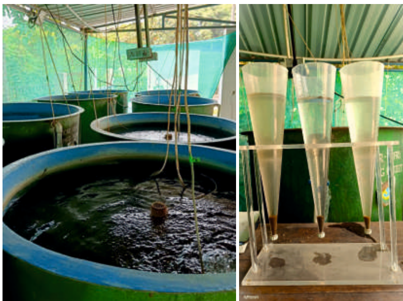
Biofloc tanks and Imhoff cone indicating the floc volume
